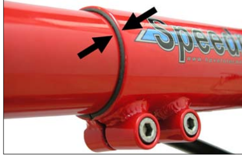
The plastic bush between front boom and main frame must be visible at all time.
