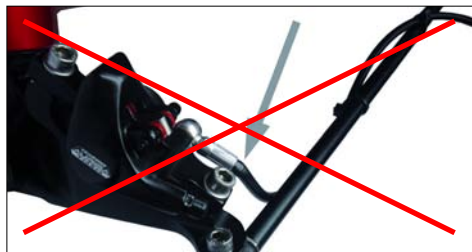
The bow of the hose is routed under the track rod: Danger of snapping off the hose (cf. arrow).
