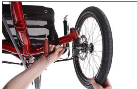
Loosen the bolt inside the locking part to remove the wheel from the knuckle.
