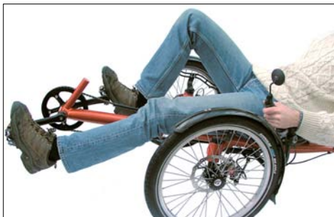
Adjust the front boom so that your knee will not be fully straightened when pedaling.
