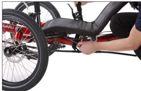
Handlebar width is adjusted at the stem clamp under the seat.
